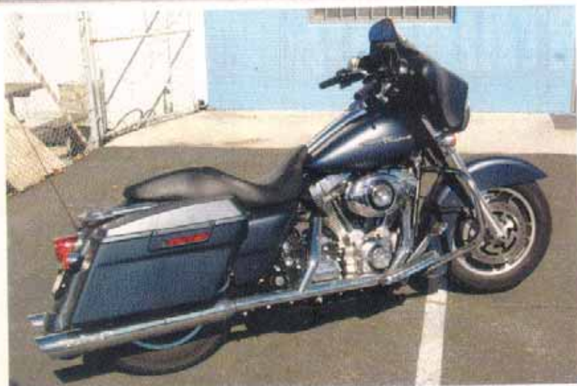
1. The bike we had the pleasure to ride with the 131-inch engine was an '08 Street Glide. This model featured the throttle-by-wire EFI unit; consequently, the stock EFI unit was used on the engine, which somewhat limited the power output due to the throat size.
