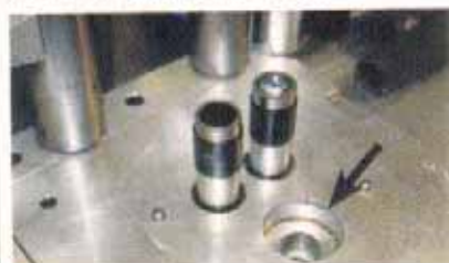
5. One of the first operations is the installation of the inner camshaft bearings into the right crankcase. Here the needle bearings were placed on these two stands and the case was pressed down onto the bearings. The hole in the table (arrow) is for the pinion shaft of the flywheels for the next operation.
