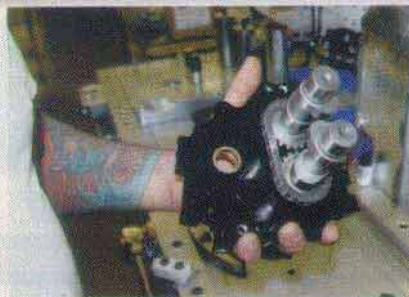
15. The camshafts come pre-assembled using the cam grind specified for the size and output of the engine—the cam plate is a JIMS billet item.
