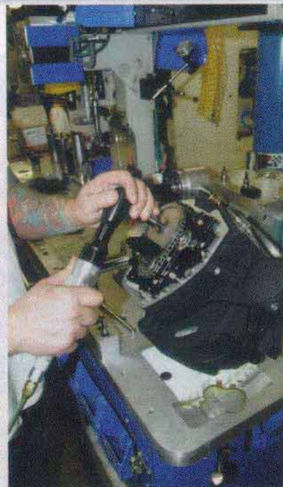
17. The camdrive chain assembly was installed and then torqued followed by a hydraulic chain tensiometer.
