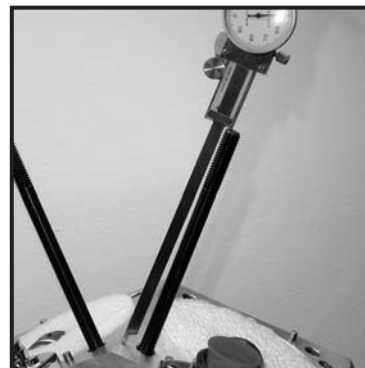
Fig.13- Measure stud height
