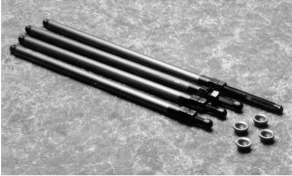
1. Although the pushrod seats may be changed without removing the tappets from the tappet blocks, JIMS suggests removing the tappets for inspection and cleaning. Check all rollers. If bad replace with JIMS Tappets No.2459-1, No.2460-1, or 2461-1.
